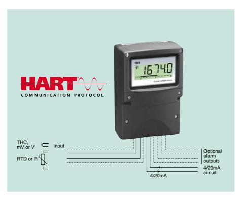
**The new BA674D** is a second generation, loop powered indicating temperature transmitter which replaces the BA574C. It provides an accurate local digital temperature display, plus a 4/20mA output, which may be scaled to represent any temperature range. Incorporating new facilities such as HART<sup>®</sup> digital communication and a robust GRP enclosure with a separate terminal compartment, the BA674D remains electrically compatible with the earlier model.
